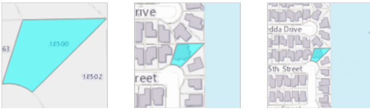
Feature maps with a buffer distance of 0 (left), 50 m. (center), and 100 m.
